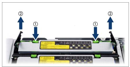
Figure 34: Example: Removing memory board
